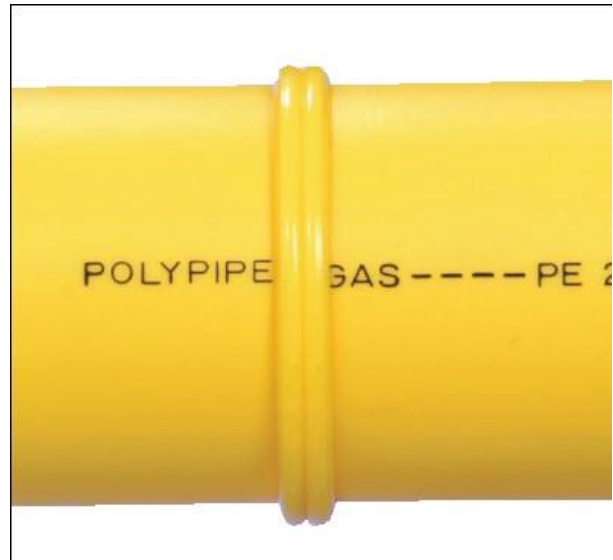
Melt bead too large due to excessive heating and/or over-pressurizing of joint.
