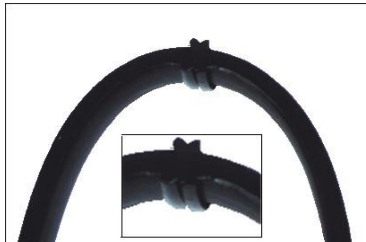
Bend back testing. No gaps or voids.
