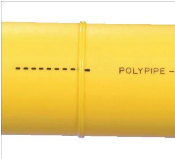
Melt bead too small due to insufficient heat time.
